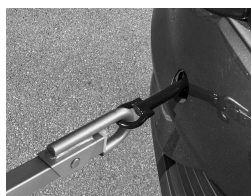
Figure 1: Connecting the vehicles
