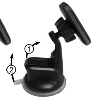
Fig. 9: Detaching the smartphone holder
