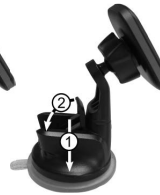
Fig. 8: Pressing and closing the locking lever
