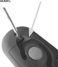
Figure 2: Opening the battery compartment
