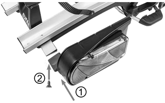
Figure 1: Installation of the rear lights
