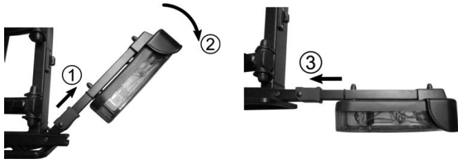
Figure 12: Locking the light mounts
