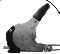
Figure 3: Tensioning the belt
